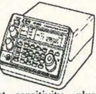
Extreme coverage, excellent sensitivity, plus processor controlled band pass filtering and attenuation to eliminate interference. Top rated receiver in its class, offers AM, NFM Wide FM, LSB, USB, CW modes. RS232 control. Lockout in search. 4 priority channels. Delay & hold & Freescan modes. AC/DC pwr cord and whip ant. included. Size: 3 1/7H x 5 2/5W x 7 7/8D. Wt 2lbs., 10oz. Fax fact document #105.
